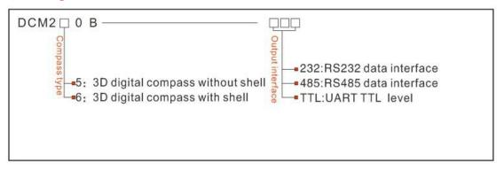
E.g: DCM260B-232: 3D with enclosure sealed/RS232 output
